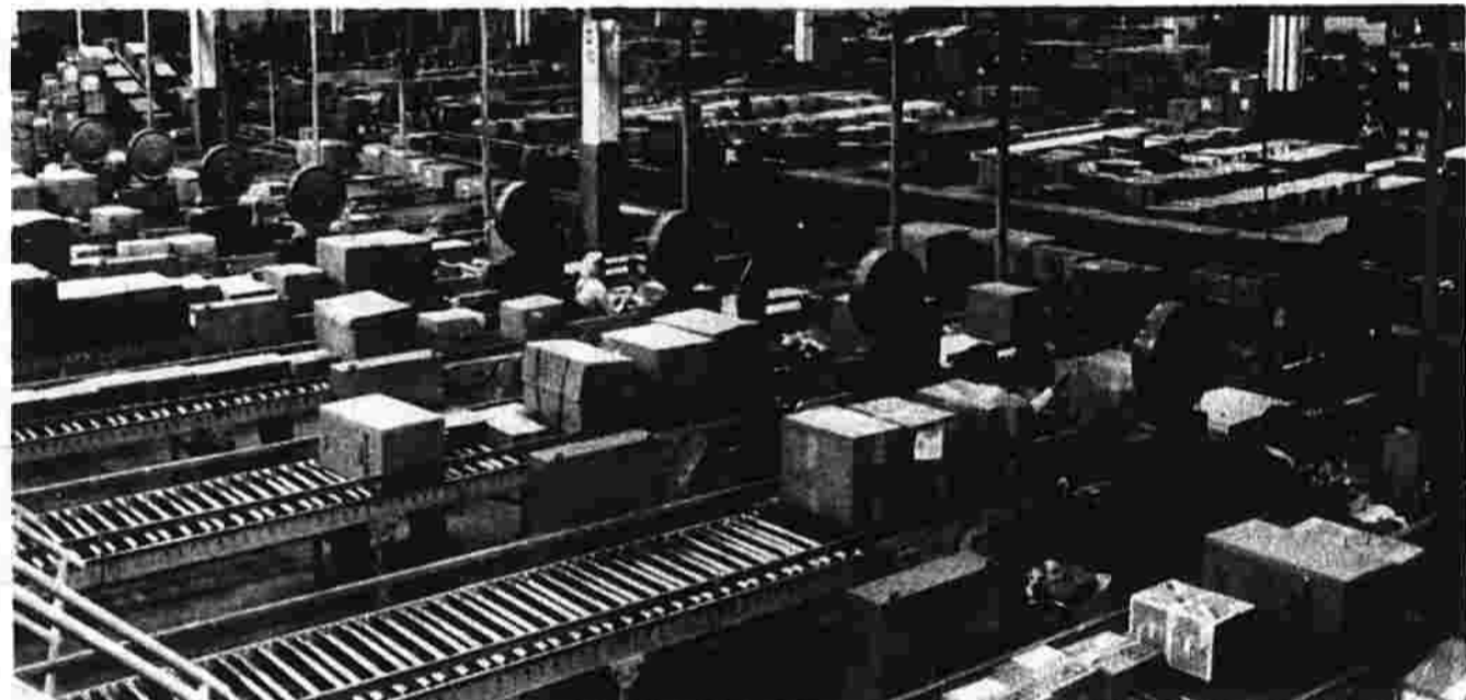
A computerized checking system weighs all incoming packages for inventory purposes. If the package weighs the proper amount, it is sent by conveyor belt to the storage area.
